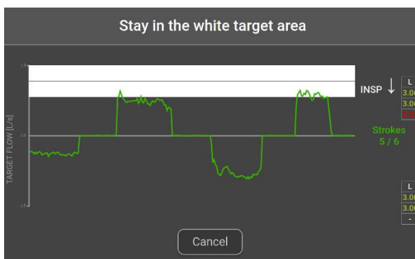
Figure 26 - Example of flow tracing during the slow spirometry volume verification
