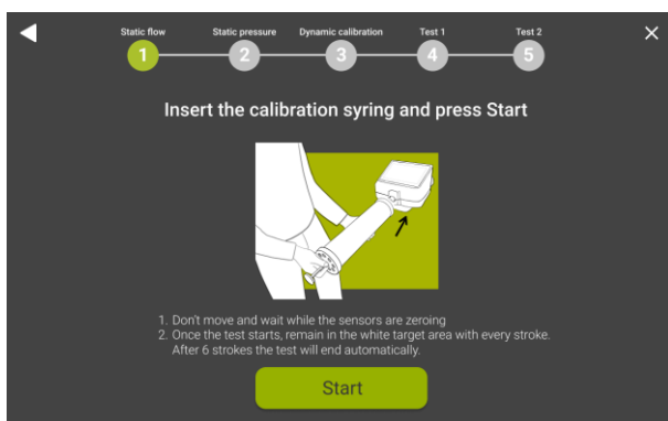
Figure 25 - Instructions for the Slow Spirometry volumes verification
