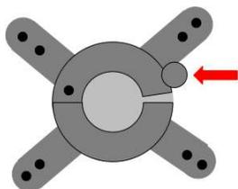
Figure 8 - VESA connector, the arrow indicates the safety locker that should be properly engaged to guarantee a secure connection between the device and the holder
