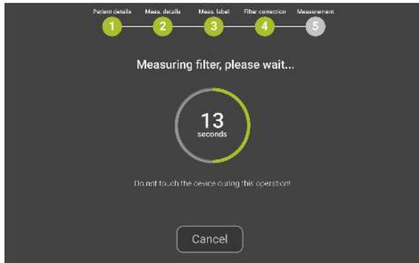
Figure 49 - Sensors auto-zeroing and filter impedance measurement
