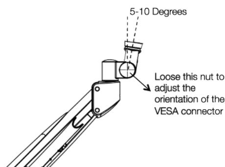
Figure 7 - Adjust the orientation of the VESA connector
